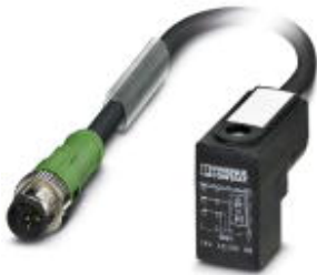
Sensor/Actuator cable, 3-position, PUR, Black-gray RAL 7021, Plug straight M12, on C valve plug (8 mm), Cable length: 0.3 m
