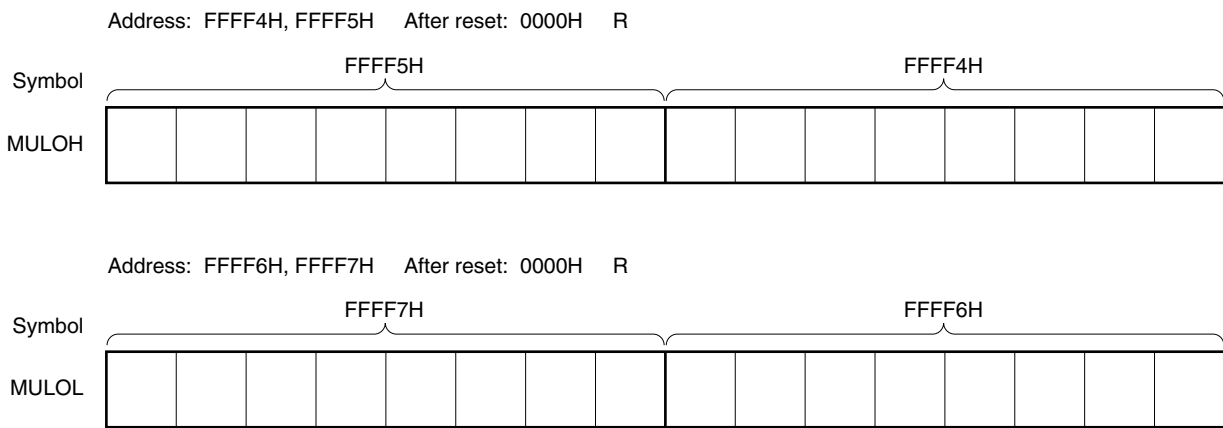
Figure 14-2. Format of 16-bit higher multiplication result storage register and 16-bit lower multiplication result storage register (MULOH, MULOL)
