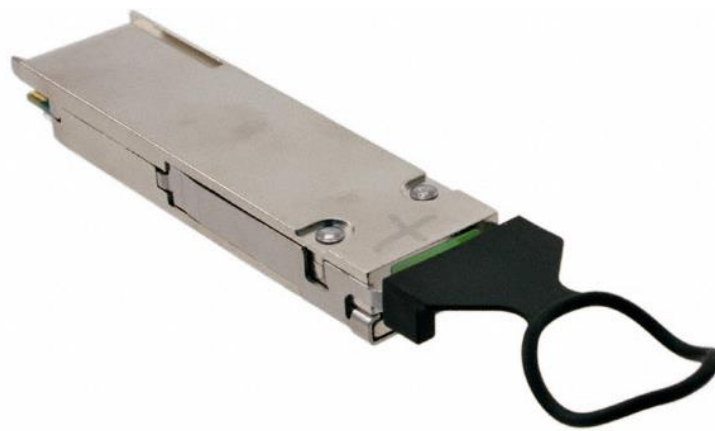
Figure 8-2 QSFP+ Loopback Fixture
