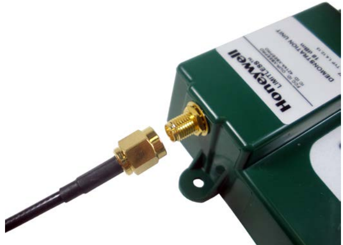
Figure 13. Limitless™ WDRR RP-SMA Connection, Remote
